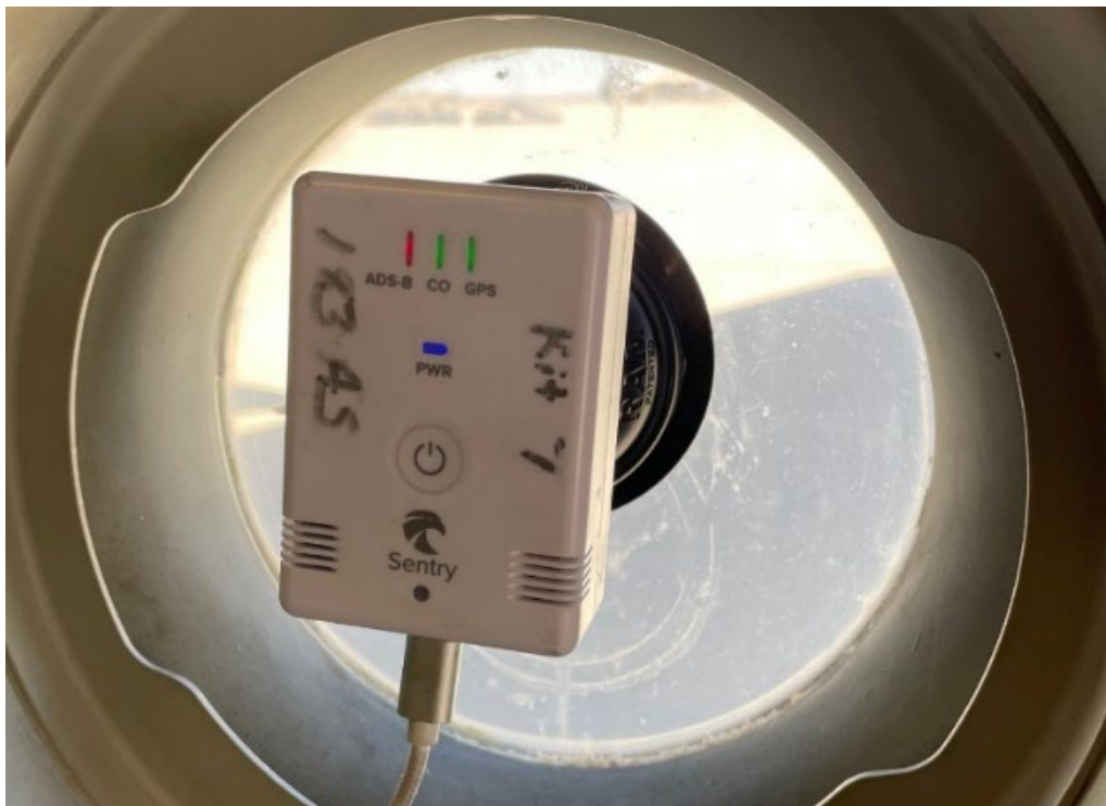
Figure 3: A portable tri-constellation GNSS receiver aboard a USAF C-17 (author photo)
